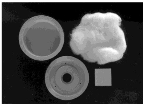
Figure 1. Components of the flow-through device: (upper row, from left to right) plastic bottom member and absorbent material; (lower row, from left to right) plastic top member and membrane.
